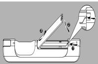
Insert 4 batteries type R03 or AAA into the remote control with the correct polarity as indicated by the "+" and "-" symbols inside the battery compartment
