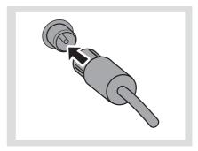
2 To improve FM reception, fit the plug of the wire antenna, as shown, into the plug of the extension line
