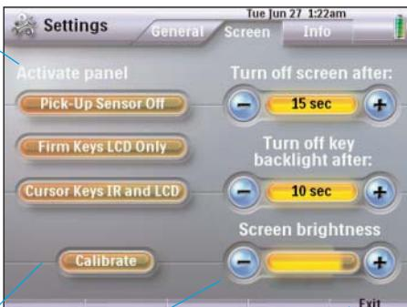
**Note** The screen is calibrated in the factory. Do not use this function unless you experience problems with the touch screen.
