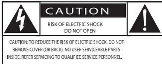
This 'bolt of lightning' indicates uninsulated material within the device may cause an electrical shock. For the safety of everyone in your household, please do not remove the covering.
