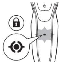
You can lock the shaver when you are going to travel. The travel lock prevents the shaver from being switched on by accident (see 'Activating the travel lock').
