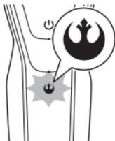
For maximum shaving performance, replace the shaving heads every year. The shaver is equipped with a replacement reminder which reminds you to replace the shaving heads. The replacement reminder flashes to indicate that you have to replace the shaving heads. (see 'Replacing the shaving heads')
