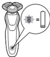
When the battery is almost empty, the bottom light of the battery charge indicator flashes red.
