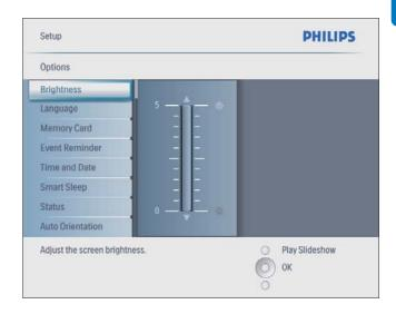
3 Press ▲/▼ to adjust brightness, and then press OK to confirm.
