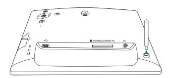
2 Screw the stand into the stand hole firmly.
