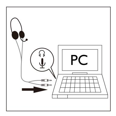
Connect the headphone plug to the  $\widehat{\mathbf{h}}$  socket and the microphone plug to the  $\widehat{\mathbf{\Psi}}$  socket of your computer.
