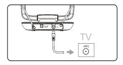
3 Connect the DC plug to the antenna and the power supply to a 230-240V AC outlet.
