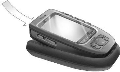
Charging starts immediately. The blue charging LEDs on the front of the docking station indicate that the battery pack is being charged.
