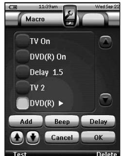
**Note** You can assign a macro to most buttons of your ProntoPro NG. Only the hard buttons on the left side of ProntoPro NG (Backlight, Page Up and Page Down) cannot be programmed.
