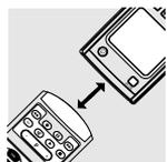
If your equipment is not included in the code list, or if specific codes on your remote control are missing, the SBC RU865 has the solution. It can copy and replicate codes from your original remote control. Here's how.. Place your original remote control facing the infra-red sensor window of the SBC RU865. Place both remote controls on a flat surface, 3-8 centimetres apart.
