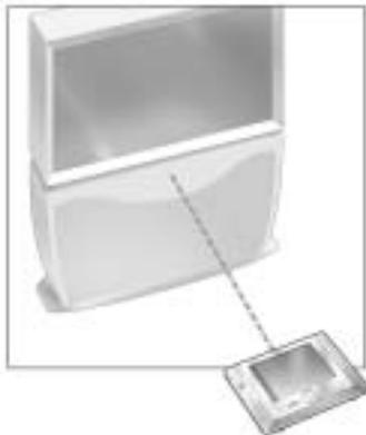
For every action the iPronto sends out a specific IR signal, called an “IR code”. The iPronto RC contains a huge database that contains numerous IR codes for all kinds of devices.
