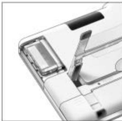
**Note** Do not install any other adapter. Do not remove the Wireless LAN Adapter when the iPronto is activated. After the Wireless LAN Adapter is installed, there is no need to remove it. It can permanently be left inside the iPronto.
