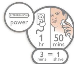
An energy-efficient, powerful lithium-ion battery gives you more shaves per charge. Charge it for an hour and you'll have up to 50 minutes of shaving time. Charge it for 3 minutes and you'll have enough power for one shave.
