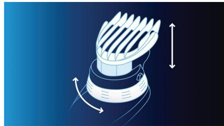
Easily select and set your desired hair length by turning the integrated zoom ring. The length settings are clearly visible on the side of the combs.
