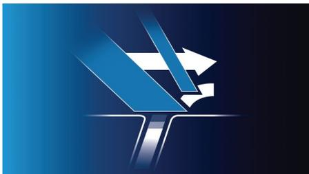
The dual blade system built into our electric razor lifts hairs to cut comfortably below skin level for a closer shave
