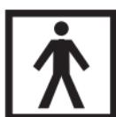
This symbol means: Philips BlueControl is specified as applied part type BF. B indicates that it is used on the Body and F indicates that it is Floating from (not connected to) the mains voltage.
