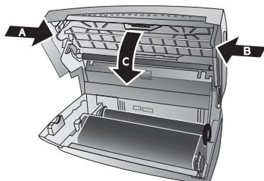
4. Lightly wipe the upper side of the scanner glass (A) and the lower side of the document feeder/scanner film (= white plastic plate) (B) with a cloth.
