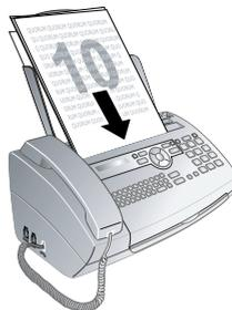
3. Set the desired resolution. You can choose between **RESOL. : STANDARD** (for documents without special features), **RESOL. : FINE** (for texts with small print or drawings) and **RESOL. : PHOTO** (for photos). Press **RES**. The configured resolution appears on the display. Press **RES** again to change the resolution.
