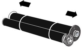
7. Place the larger roll with the ink film in the rear ink film tray. The blue gear wheel must be on the right hand side.
