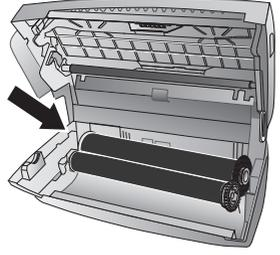
8. Place the smaller roll without ink film in the front tray. The blue gear wheel must be on the right hand side and the pin must be inserted in the depression on the left hand side.
