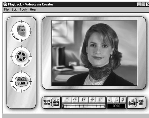
After starting the 'Videogram Creator' software, you will see the 'live' camera image. Move the camera about, adjust the lighting and turn the red lens ring to focus. You will immediately see the effect of this on your screen. Adjust the sound and image settings by clicking on 'Edit' in the menu bar and selecting the 'Video Settings' option. Consult the electronic manual on the CD-ROM for a detailed explanation of all the possible settings.
