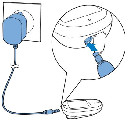
Plug the charging adapter into the headset/charging jack at the bottom of the phone.
