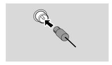
For better FM stereo reception, connect an outdoor FM antenna to the FM AERIAL (FM ANTENNA) terminal.
