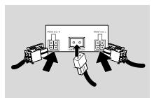
Connect the passive subwoofer to the SUBWOOFER (8Ω) terminal with the supplied subwoofer cable by matching the plug types.
