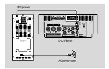
After everything is connected properly, plug in the AC power cord to the power socket.
