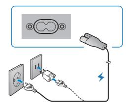
A round-to-flat power plug adaptor is supplied. If the wall power sockets are for flatpin plugs, connect the adaptor tightly to the power plug first.
