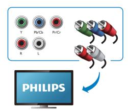
Connect a progressive scan TV through component video cables for higher quality video.
