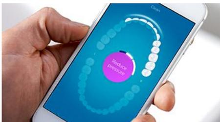
Three smart sensors send personalized brushing data to the Philips Sonicare app. Location sensor shows patients where they're brushing too little for better coverage. Scrubbing sensor helps guide patients to reduce scrubbing for optimized technique and a deeper, more gentle clean. Pressure sensor tracks brushing pressure and gently pulsates the handle to tell patients when to adopt a softer touch.
