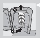
Remove the protective screen in front of the UV light bulb. To remove the screen, gently lift it up (1) and pull it out (2).
