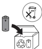
**9** Cover the battery contacts with tape to prevent any electrical short from residual battery charge. The rechargeable battery can now be recycled and the rest of the product discarded appropriately.
