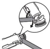
**7** Insert the screwdriver between the bottom of the battery and the black frame to break the metal tab connecting the battery to the green printed circuit board. This will release the bottom end of the battery from the frame.
