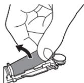
**8** Grab the battery and pull it away from the internal components to break the second metal battery tab.
