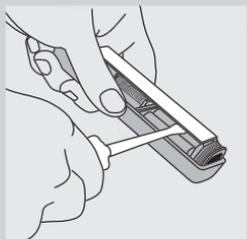
**7** Insert the screwdriver underneath the electronic circuit board in multiple places.
