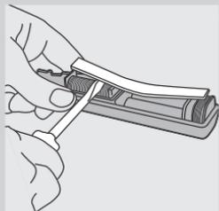
**8** Twist and pry the electronic circuit board loose until it is completely separated from the handle.
