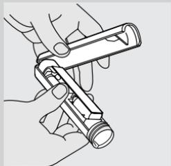
**6** Pull the 2 handle sections completely apart.
