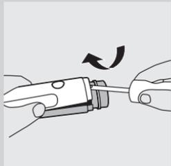
**5** Now use the screwdriver as a lever to pry the 2 handle sections apart.
