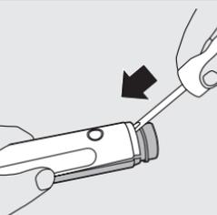
**3** Remove the screwdriver and repeat the above instruction using the other slot located on the opposite side of the handle. Twist the blade and the housing will continue to split.
