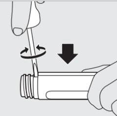
**2** Insert a screwdriver into one of the slots located near the top portion of the handle, push the screwdriver blade into the handle as far as it will go, and twist the blade. The housing will begin to split.
