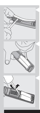
Twist and pry the electronic circuit board loose until it is completely separated from the handle.
