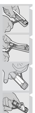
6 Insert the screwdriver underneath the electronic circuit board in multiple places.
