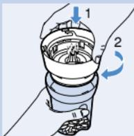
**3** Screw the blade unit onto the beaker. If this requires some effort, moisten the rubber ring with a drop of water.
