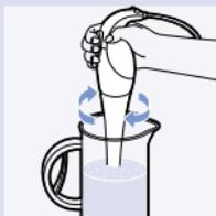
**1** Immerse the blade guard completely in the ingredients.
