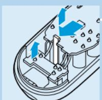
**4** Insert the screwdriver into the small slot in the printed circuit board marked with an arrow. Push the screwdriver down until parts of the printed circuit board break off.
