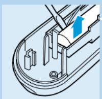
**5** Press the hook and remove the printed circuit board.
