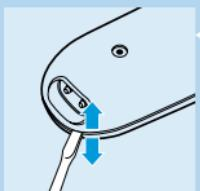
**2** Undo the screw in the housing of the trimmer.
