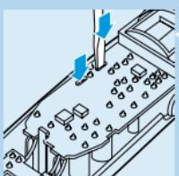
**3** Separate the 2 housing parts by means of a screwdriver.
