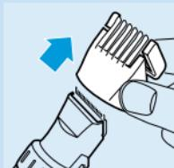
Never pull at the flexible top of the comb attachment. Always pull at the bottom part.
