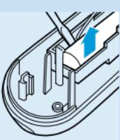
**5** Press the hook and remove the printed circuit board.
