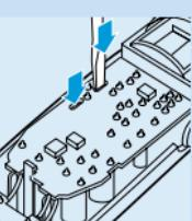
**3** Separate the 2 housing parts by means of a screwdriver.
