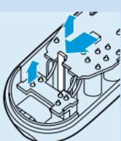
**4** Insert the screwdriver into the small slot in the printed circuit board marked with an arrow. Push the screwdriver down until parts of the printed circuit board break off.
