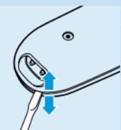
**2** Undo the screw in the housing of the trimmer.
