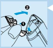
**5** To reassemble the clipper, insert the hook of the cutting unit into the housing.
