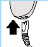
**1** Put the appliance plug into the shaver as far as the line on the plug.
