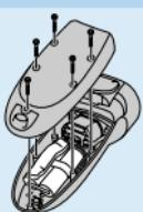
**2 Remove the batteries.**
