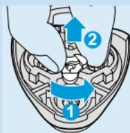
► Remove the retaining frame.
