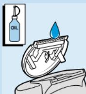
3 Lubricate the trimmer teeth with a drop of sewing machine oil every six months.
