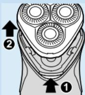
**3** Press the release button and remove the shaving unit.
