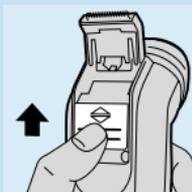
**1** Open the trimmer by pushing the slide upwards.
