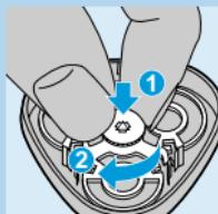
**7** Reassemble the shaving unit by replacing the retaining frame. Press the wheel and turn it clockwise.
