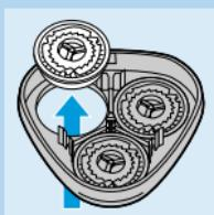
**4** Remove and clean the shaving heads (cutters and guards) one by one.
