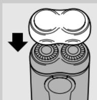
► Put the protection cap on the shaver to prevent damage.
