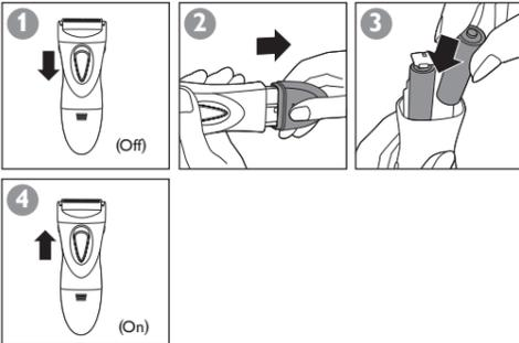
NOTE: Make sure the (+) and (-) markings on the ends of the batteries match those inside the battery compartment.
