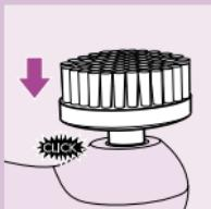
**1** Push the cleansing brush onto the connection pin until it locks into position with a click.
