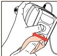
*To clean the rollers, select Level 1, cover the suction opening with your thumb so that the rollers start to rotate, then wipe the rollers clean with a damp cloth, as shown.*
