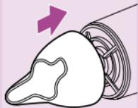
► To concentrate the airflow, you can connect the concentrator to the air outlet.
