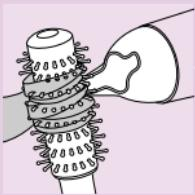
► The concentrator allows you to direct the airflow straight at the brush you are using to style your hair.
