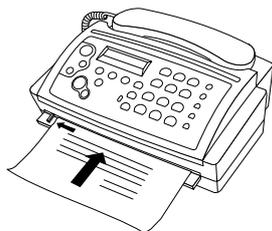
Take the first page of the document and place it **face up** as shown in the picture. Slide the document into the fax along the document guide on the left hand side of the feed slot until it stops. Wait for a moment: The document will now be slightly drawn in automatically by the feeding mechanism. Once the document has been drawn in by the feeding mechanism, it should not be pushed in any further, otherwise the top part will be missing when you make a copy or transmit a fax.
