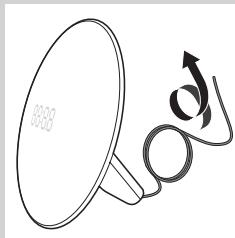
*Tip: Fully unwind the antenna to use the radio function.*
