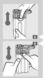
1 Press one of the release buttons at the side to remove the top of the carafe as shown in the figures (A or B).
