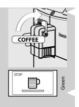
2 Push the lever upwards to select the "COFFEE" function.
