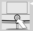
■ Turn off the machine by pressing the "()" button. Wait until the "()" button blinks and unplug the power cord.
