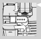
3 Slide the milk carafe dispenser to the right up to the " 📥 " icon. Make sure that the dispensing spout handle is perfectly aligned to the icon " 📥 ".
