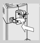
1 Slightly tilt the water dispensing spout and insert it all the way in into the guides of the machine.
