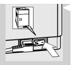
2 Switch the power button to "I" to turn on the machine. The "()" button blinks.
