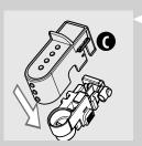
6 Detach the lid (C) from the milk carafe dispenser by pushing downwards while slightly pressing on the sides.
