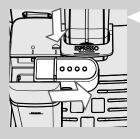
Slide the milk carafe dispenser to the right up to the " A " icon. Make sure that the dispensing spout handle is perfectly aligned to the icon " " "."
