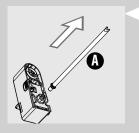
4 Remove the suction tube with the fitting (A) from the milk frother.
