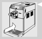
14 Insert the coffee grounds drawer with the drip tray back into the machine and close the service door.
