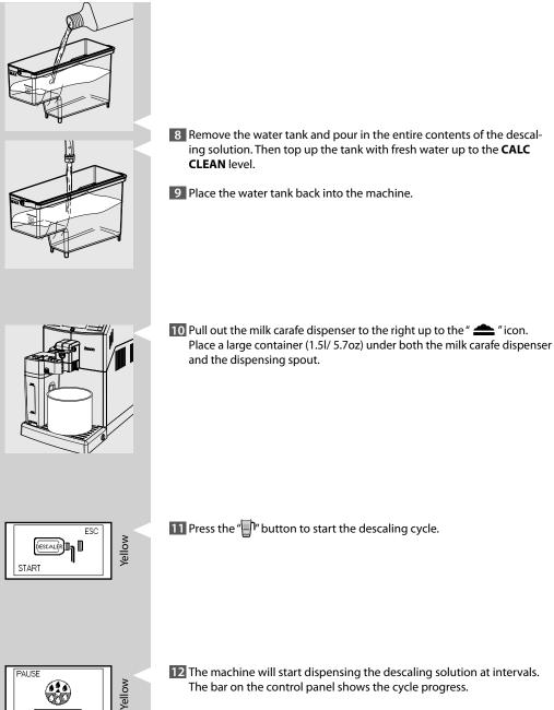
The bar on the control panel shows the cycle progress.
