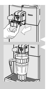
Remove the lower part of the dispensing spout to allow a tumbler to be used.
