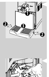
**2** Raise the dispensing spout and remove the drip tray and coffee grounds drawer by pressing the side buttons. Only at this time open the service door.
