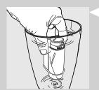
2 Remove the "INTENZA+" water filter from its packaging, immerse it vertically (with the opening positioned upwards) in cold water and gently press the sides so as to let the air bubbles out.
