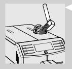
3 Lift the pre-ground coffee compartment lid and add one measuring scoop of pre-ground coffee to the compartment. Use only the measuring scoop supplied with the machine. Then close the pre-ground coffee compartment lid.
