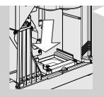
12 Insert the coffee residues drawer into its seat and ensure that it is correctly in place.
