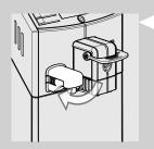
2 Push the water dispensing spout towards the bottom while rotating at the same time, until it is locked in the machine as shown in the figure.
