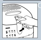
1 Lift the basket handle to locked position to raise the wire basket to its highest position.
