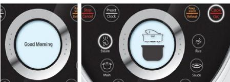
Each cooking program will come with step by step visual and audio guidance during set up and cooking. User can simply follow the instructions shown on the screen. It provides four language settings options for text guidance.
